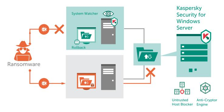
In addition to **detection**, there is a prevention mechanism in Kaspersky Security for Windows Server. While SMB/CIFS protocols can't give us information about the process on the ransomware's host, we can obtain the host's IP address. **Host Blocker** technology can then prevent this infected host from engaging in any further activity with shared folders.
